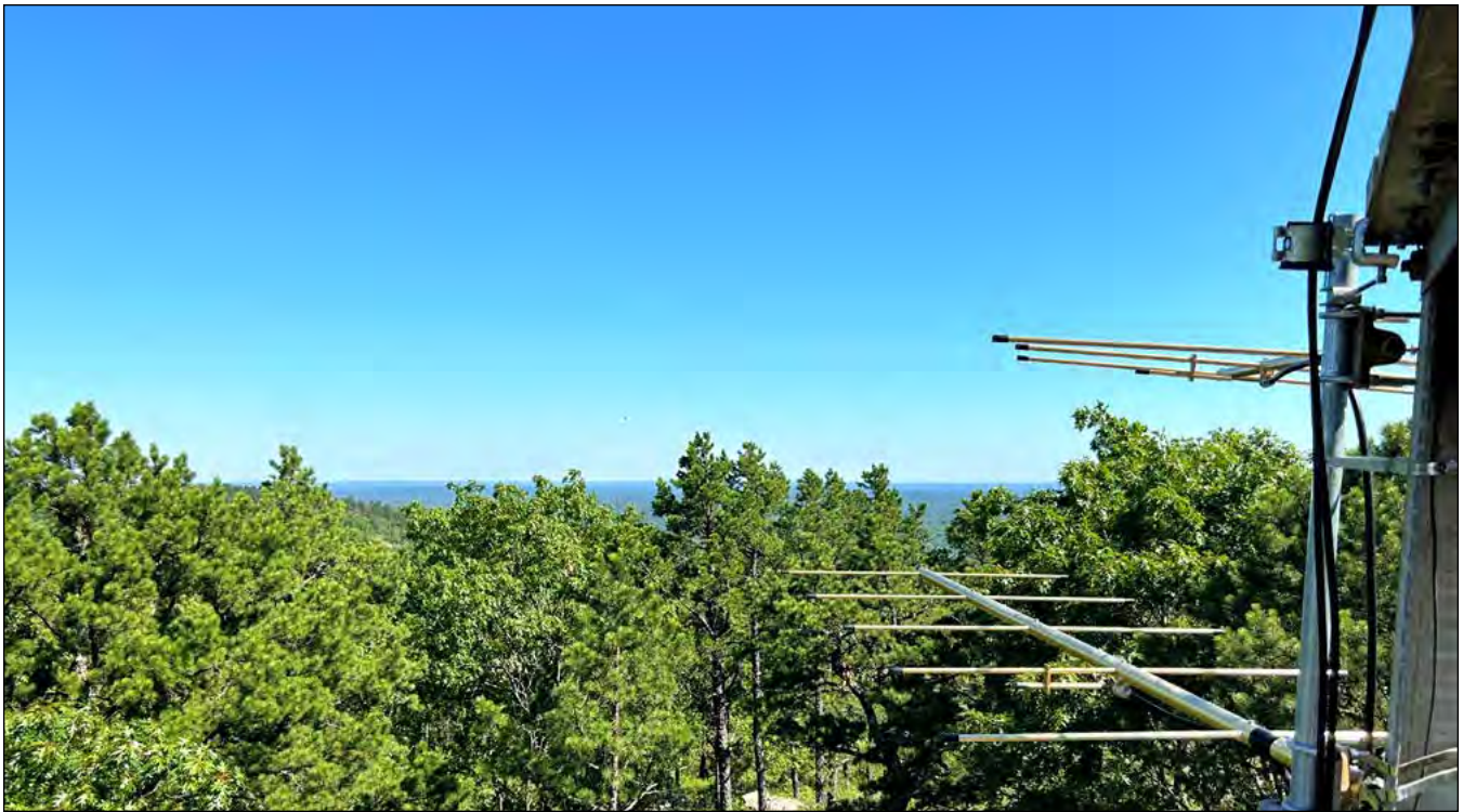
Figure 2. Motus stations like this one at Stegall Mountain Natural Area in Missouri use antennas to detect the signals emitted from Motus tags attached to birds within range of a station.
